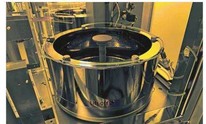
Solvent module for lift-off or resist strip for standard solvents and various lift-off techniques
