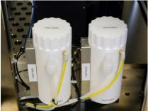
The system consists of a sensor-controlled reservoir and a suck-back dispense valve. The reservoir supplies the dispense valve which is mounted near the nozzle. The resist volume is set by pressure and trigger time.
