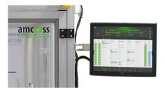
// Our intelligent ams PLOT software also controls processes in the amv 200 and is being used to write recipes. As standard, a rotatable industrial PC with touchscreen and SECS/GEM interface is used to operate the machine.
