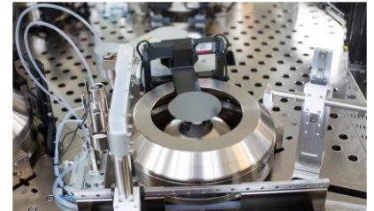
// Coater module with servo-controlled single-nozzle positioning arm, EBR, and exhaust
