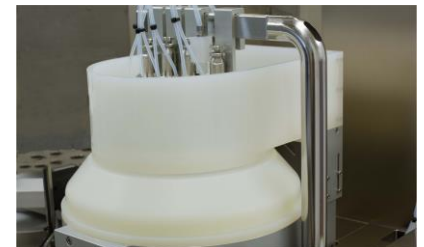
// Developer module with high splash ring for spray and puddle developing.
