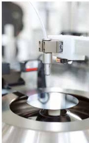
Solvent module for lift-off or resist-strip with innovative positioning arm with single-nozzle grip. Only one nozzle at the time is being carried, which holds two major advantages: on the one hand there is no particle build-up caused by friction because only one tube at the time is being moved. On the other hand, all nozzles not required for the moment remain within the drip pan which prevents the tip of the nozzle from drying out and impedes delayed dripping onto the substrate.
