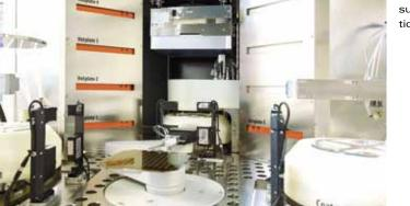
Modular, flexible and therefore alterable design of the processing surface on one of 3 basis platforms with customizable configurations and applications.
