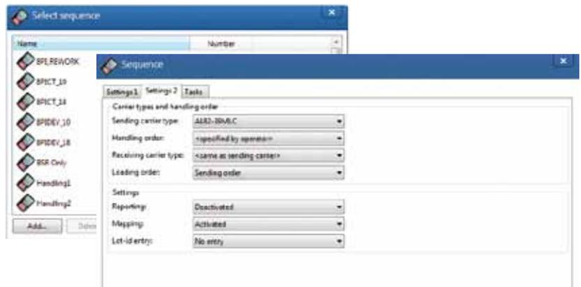
// **Integrated scheduling:** The scheduling function very precisely controls the whole process cycle and the course of the individual sequences. The aim will always be an ideal process flow and a maximum possible throughput. In addition, manual sequence-optimization is possible; e.g. for desired delays. Unique and very clever is the amc scheduling table which visualizes all processing steps.
